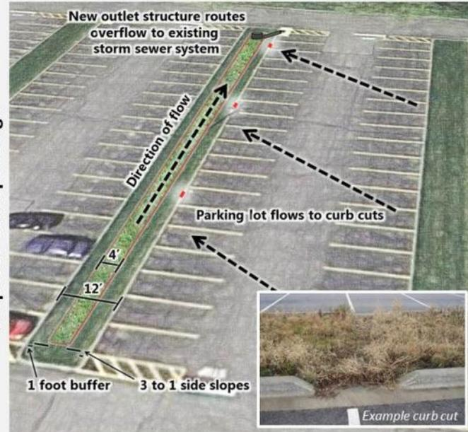
**Retrofit Description:** Ten existing grassed medians will be converted to bioretention areas. Depressions will be 1 foot deep maximum, allowing 6 inches of ponded water. Runoff will be routed to bioretention areas through new curb cuts. New outlet structures will be used to connect bioretention areas and existing catch basins. A planting plan that is prominently herbaceous native plants that are water tolerant is recommended. Costs assume volunteers planting the vegetation.
